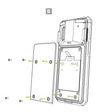
5. Align the screw holes of the Pistol Grip Adaptor with the screw holes of the SKXPro. Use the four (4) included screws to attach the Pistol Grip Adaptor to the SKXPro. (E)
