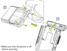
2. Slide the XCover Pro into the SKXPro and flip the top cover forward as shown. (C)  $% \left( C\right) =0$
