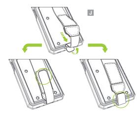
Flip the top cover back. After placing the sliding pad on the XCover Pro screen as shown in the figure, remove the XCover Pro by pushing up the sliding pad with both fingers. (H)
