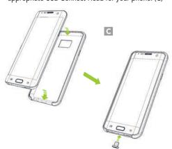
Remove the Removable Accent Plate from the back of the uniVERSE Case. Align the case with the KBCC Adaptor and slide down until you hear a click indicating it is in place. (D)
