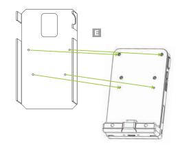
7. Screw four (4) BH M 1.7x6.0L screws into the hard plastic outer shell of the phone case to attach it to the GUA (F).
